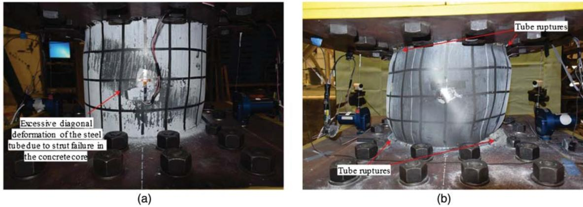
**Fig. 8.** Deformation of RCFST shear specimen (SH1R shaft 6#4, #3@7.62 cm): (a) after reaching maximum strength; and (b) specimen failure.
