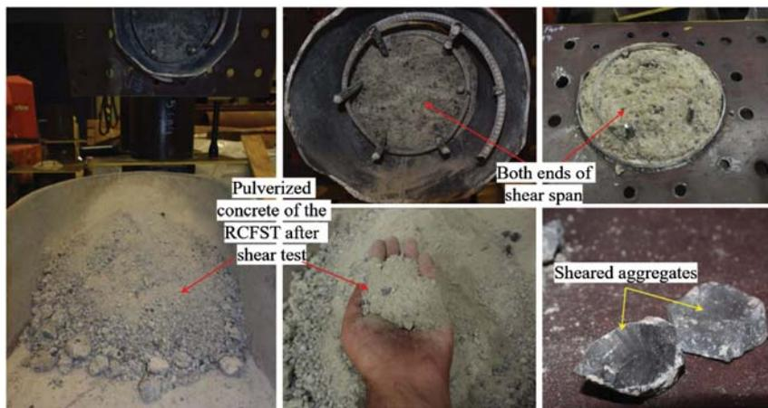
**Fig. 9.** Infill concrete state after shear test.
